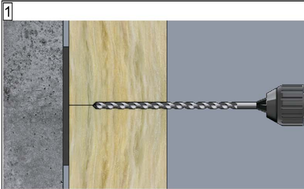
1 Drill the hole
